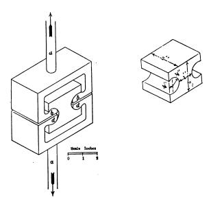
Fig. 9.—Method of making test in tension at right angles to grain. Specimen  $2^{\prime\prime}\times2^{\prime\prime}\times2^{1/2}^{\prime\prime}.$
